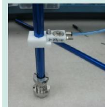
The CVT-P-10 miniature turbine vibrator enables non-stop production of 1 million INSORB Staples per month. To date, Incisive Surgical has manufactured 20 million of these fasteners.
